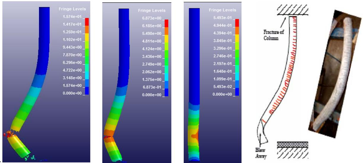
Figure 3. Sequence of Failure in Test 7
