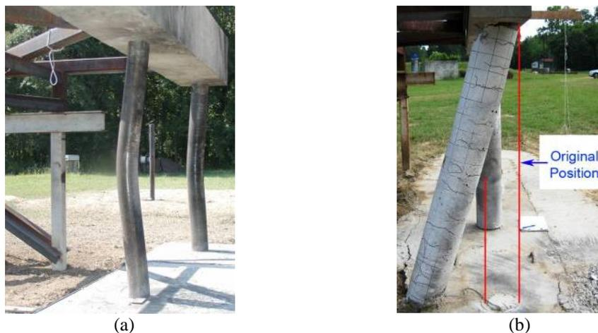
Figure 1. (a) CFST column ( $D = 127$  mm) after the test; (b) RC column after the test
