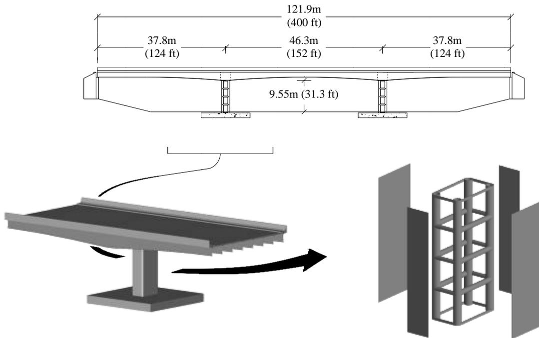
Figure 5. Final multi-hazard resistant bridge pier concept
