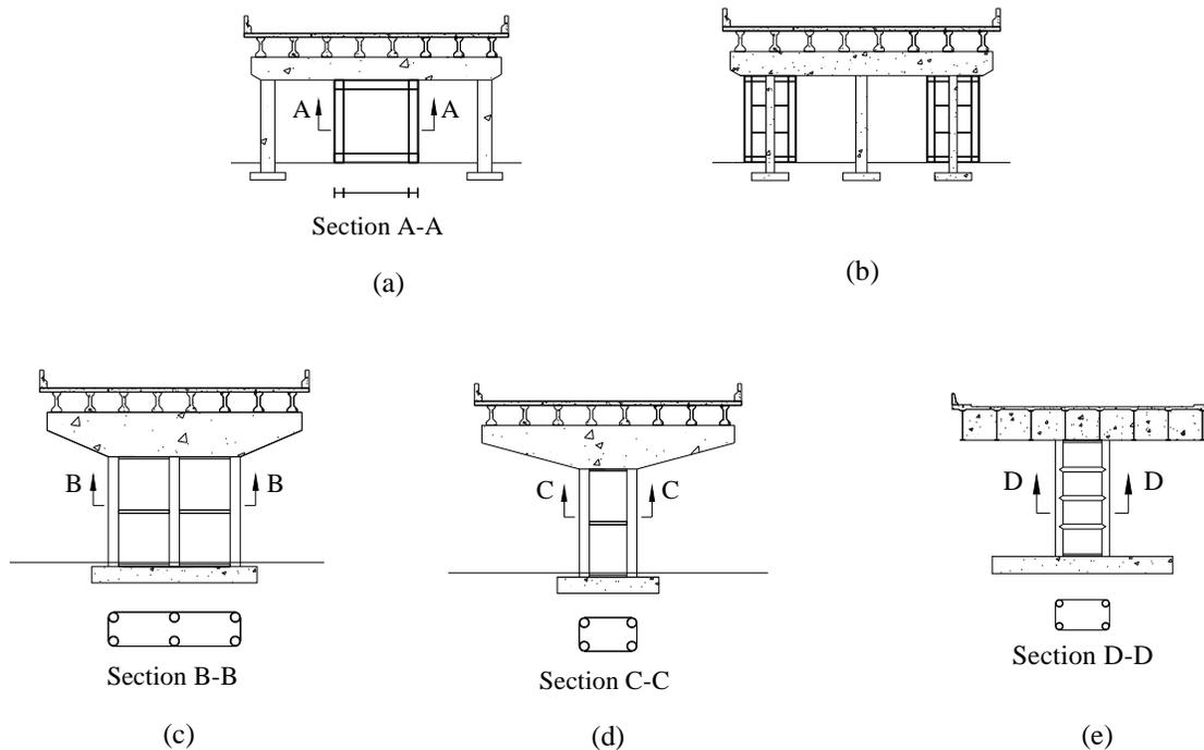
Figure 4. Progression of multi-hazard resistant SPSW bridge pier concept
