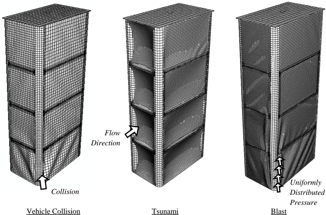
Figure 7. Finite element model following analysis for vehicle collision, tsunami and blast
