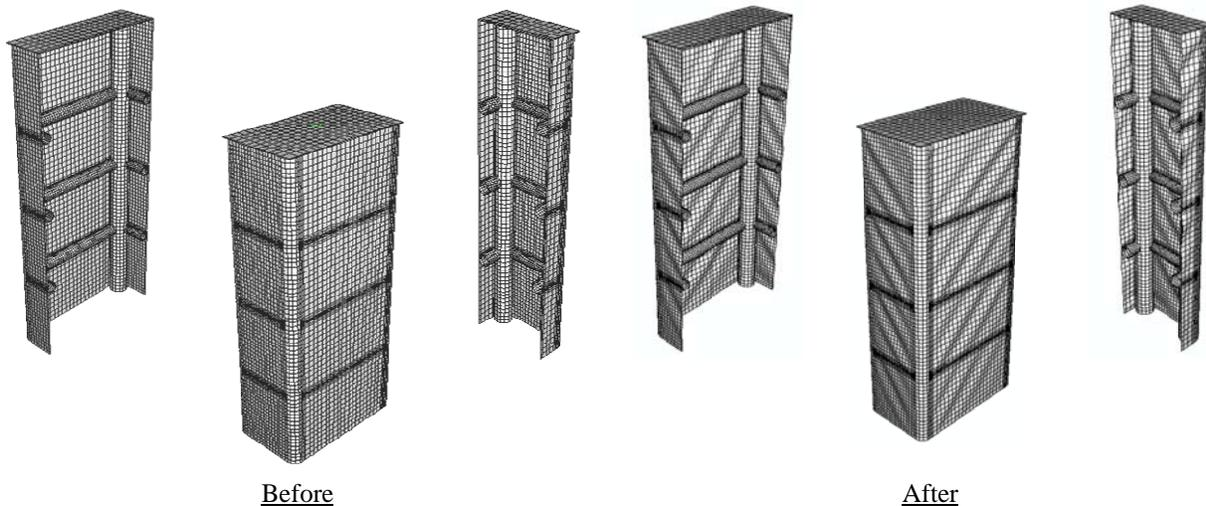
Figure 6. Finite element model before and after the pushover analysis
